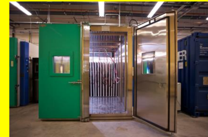
CFV Labs Chamber: -40°C → +85°C
