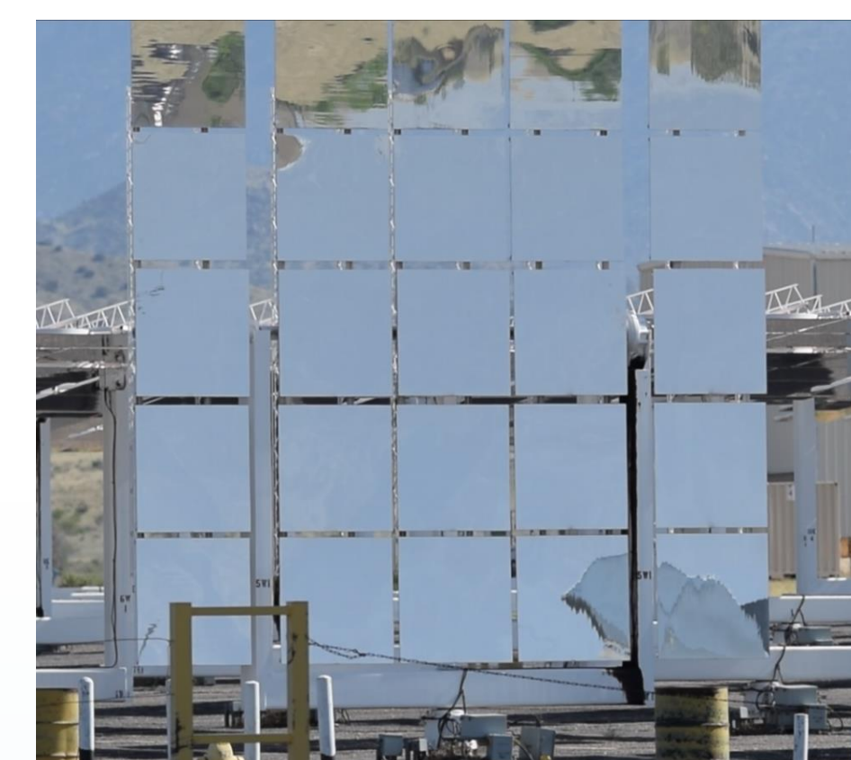
Multifacet heliostat measured by SOFAST
