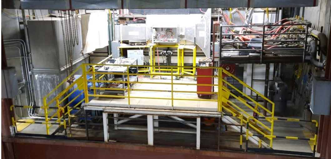
Materials test level with high speed (<0.5 s) shutter system and 0.3 Mach wind tunnel. Water-Glycol cooled calibration panel located at the same level.
