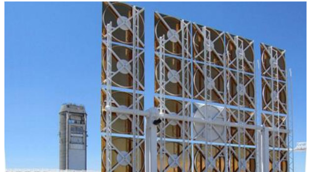
Figure 16: Hoop backing at Sandia National Solar Thermal Test Facility [i]
