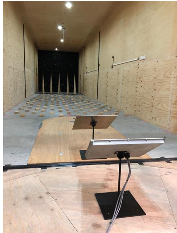
Figure 20: Atmospheric boundary layer wind tunnel heliostat testing, University of Adelaide [m]
