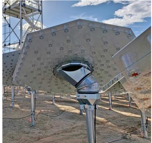
Figure 14: Heliogen pentagonal heliostat with spot supports [g]
