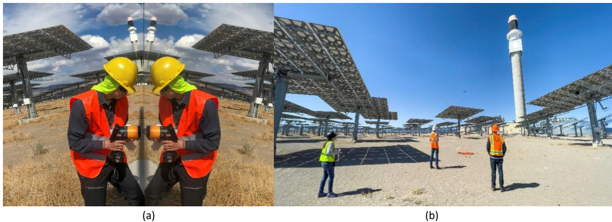
Figure 30. (a) reflectometer measurement. (b) field drone measurements for BCS target
